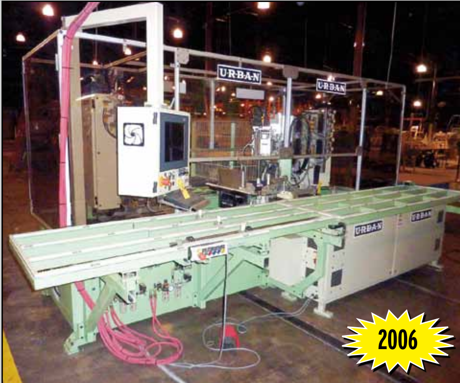
URBAN SV354 CNC WELD SEAM CORNER CLEANER
